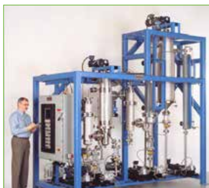
Two stage 9" and 12" WFS plant
