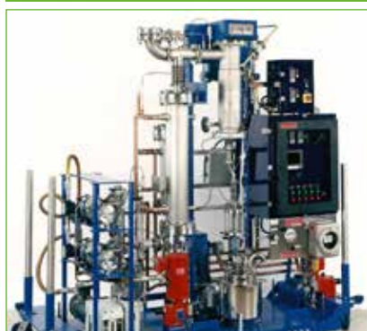
6" Hastelloy jacketed WFE pilot plant
