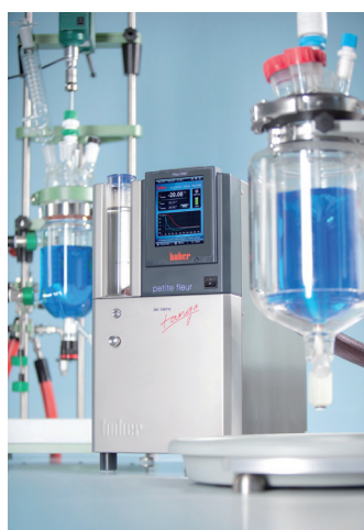
Figure 5: Unistats are in use in many industries –particularly in reactor temperature control.
