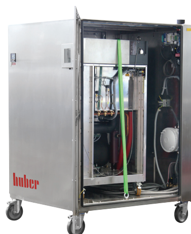
Figure 15: Ex-p Pressurised cabinet for use within hazardous areas in ATEX zones 1 & 2.
