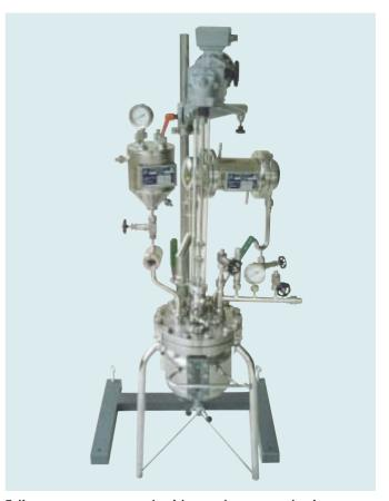
5 litre pressure vessel with condenser and stirrer drive
