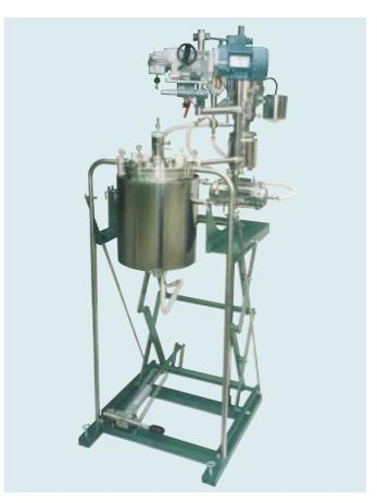
10 litre insulated vacuum vessel with lifting stage and thermostat.
