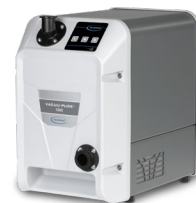
VACUU-PURE 10C Screw pump 9 m³/h, 5 \times 10^{-3} mbar Vacuum connection: Small flange DN 25
