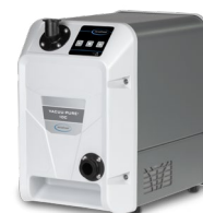
VACUU-PURE 10C Screw pump 9 m 3 /h, 5 x 10 -3 mbar Vacuum connection: Small flange DN 25
